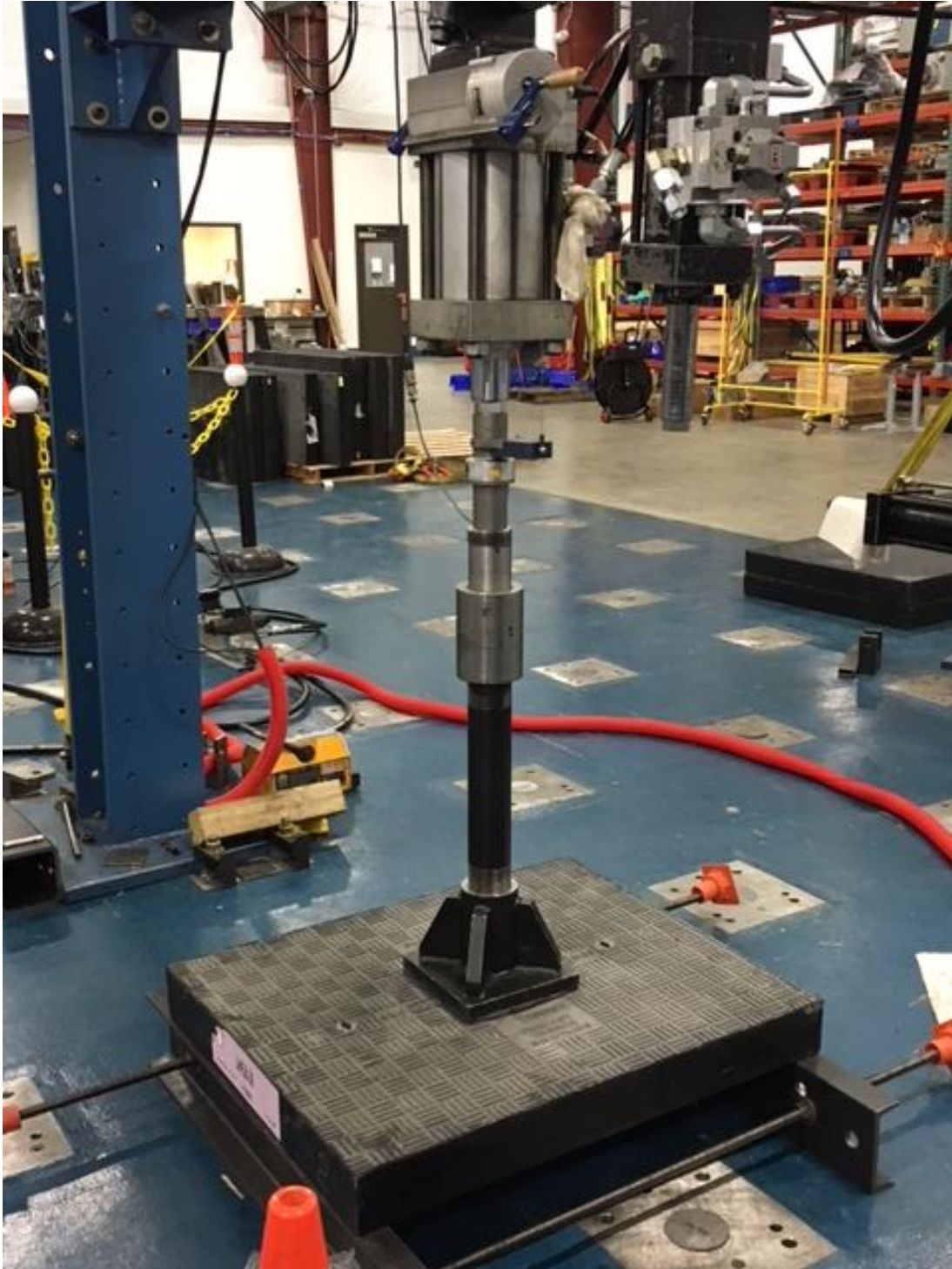
Typical Trench Cover Test Assembly
